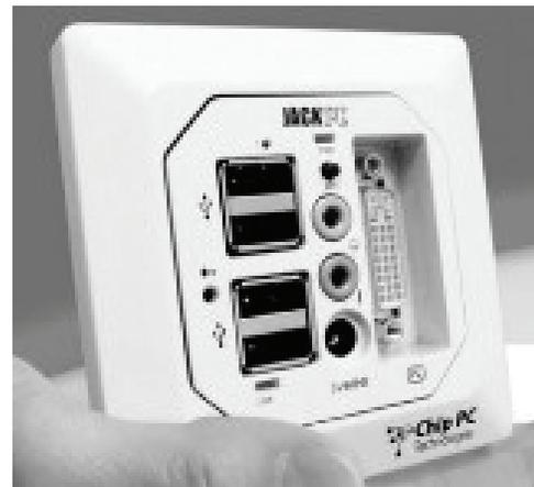
*The RISC processor is not PC compatible but does run a version of Linux and should be able to run some other operating systems. It is capable of driving two monitors at the same time and also has built in wi-fi wireless networking. In the picture below [see original online article], you can see several monitors and keyboards on a desk, all apparently plugged into power outlets. However, the so-called power outlets are actually the computers.*
